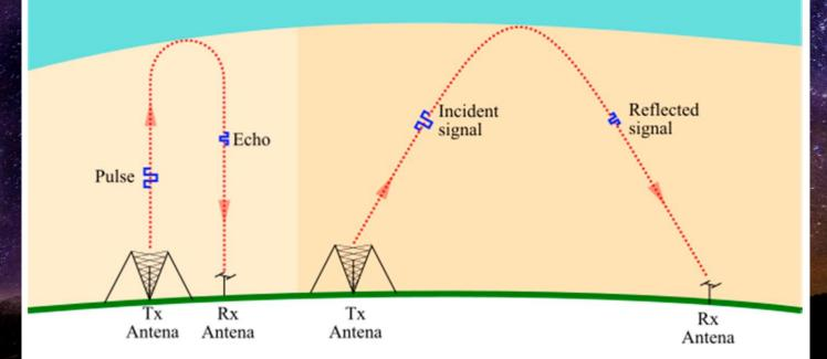
Measures of time required for signal to return to estimate high of ionised layers
