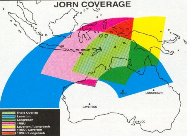
**OTHR** provides surveillance of Australia's northern coast using the ionosphere
