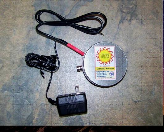
Stanford University runs a Sudden Ionospheric **Disturbance** (SID) program to detect solar flares and other ionospheric disturbances
